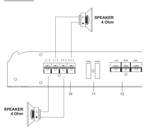
**NOTE!** The XA-5001 and XA-8001 are not designed to work in a bridged or strapped configuration. Attempting to apply these configurations will damage the amplifier and will not be covered under warranty.
